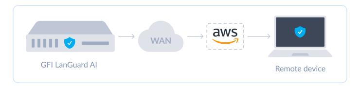
The WAN agent and the LanGuard console will communicate securely using AWS to send/receive the commands for scanning and patching. The ports used by the WAN Agent are 443, 8443, and 8883
